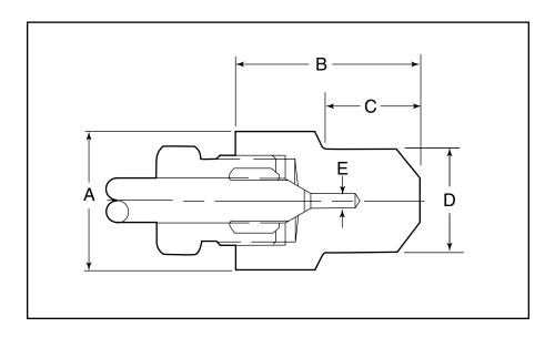
Gland and collar supplied with high pressure connections.
