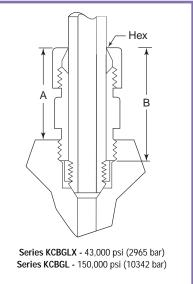
Standard Autoclave Engineers collar not included in complete assembly
