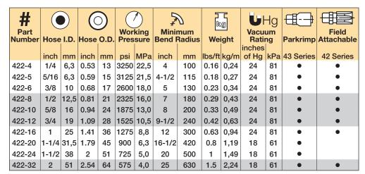
Application: Petroleum base hydraulic fluids and lubricating oils. Inner Tube: Synthetic rubber. Reinforcement: One braid steel Cover: Synthetic rubber.
